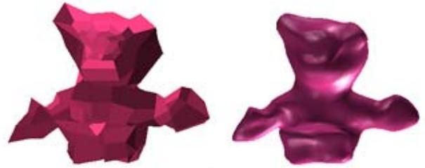
**Figure 5. Left: The mesh used to specify the connectivity and geometry of the surface patches. Right: The resulting surface.**
