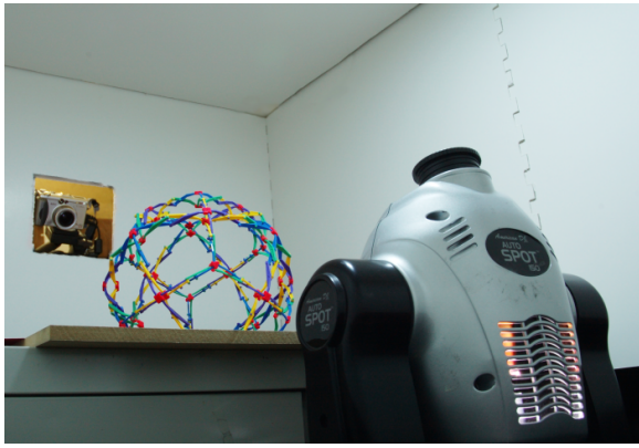
Fig. 3. The disco-light setup. The object and disco light are both enclosed in a white foam box, with the camera looking in through a window in the enclosure wall farthest from the light.
