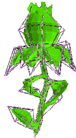
Figure 16: The polyhedral sketch for the flower. The light blue polygon (drawn in wire-frame) is built by the user. The green polygon is the dual of the first subdivision surface of the light blue polygon and is constructed automatically. The locations of the vertices of the green polygon have been adjusted to produce finer detail.
