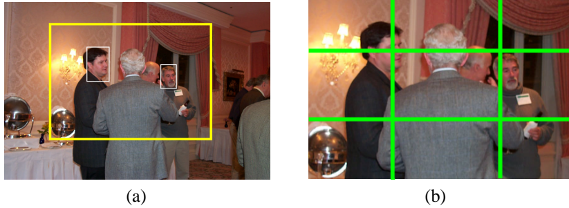
Fig. 5. Framing an image. (a) Optimal framing (large box) of the two detected faces (small boxes). (b) Optimal framing, with the rule-of-thirds lines.
