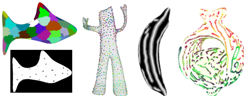
Fig. 10. From left to right: Equal area regions, distributing points across the surface, and lines that follow principle curvature directions.
