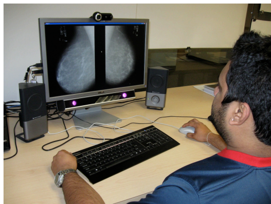
Figure 1: Photograph of experiment setup. The eye-tracking hardware is fixed to the bottom of the screen. Participants were asked to identify irregular regions in a sequence of mammogram images. Gaze manipulation techniques were used to influence their sequence of fixations during the experiment.
